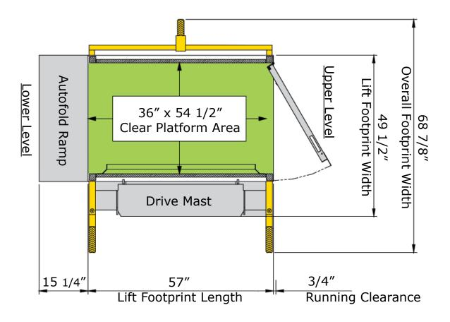
NOTE: The Genesis Staage is not intended for permanent fixed installation.
